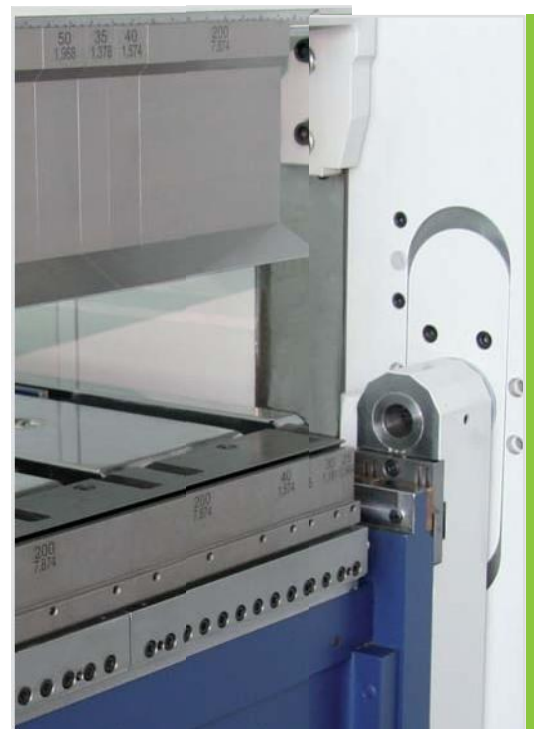
The motor-driven lowerable folding beam and the motorized folding centre adjustment are included in the standard version.
