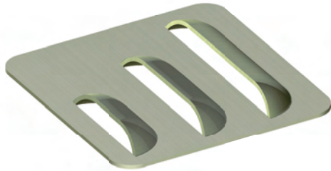
M15 CONTINUOUS RADIUS BACK LOUVER SHEARING & FORMING
