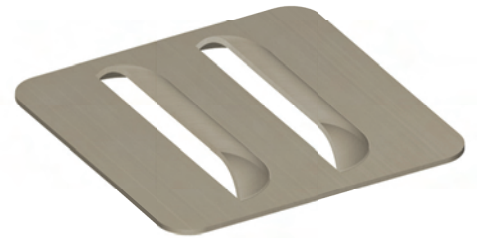
M12 RADIUS BACK LOUVER SHEARING AND FORMING
